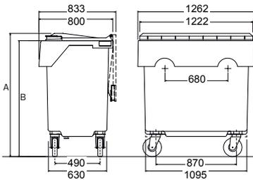
EUROPLAST mobile waste container made of HDPE for easy collection in one-man businesses. The self-centering Diamond containers allow for the quick reception of the container and provide a fixed seat by perfect latching and thus more safety. Four wheels with braking system, available with special insertion solutions.
